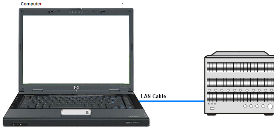
Figure 2 Connecting the PC LAN cable to the instrument LAN (cross-over cable)
